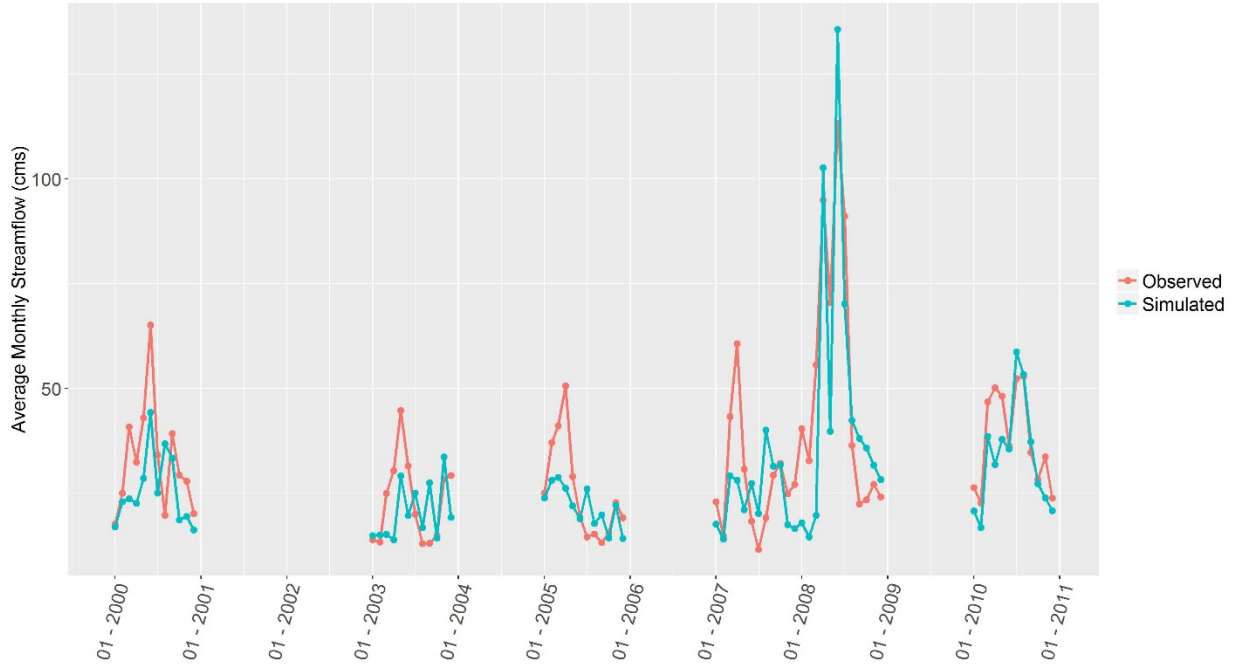
Figure D- 23. Monthly streamflow validation hydrograph for USGS site 04073500 (Fox River at Berlin, WI).
