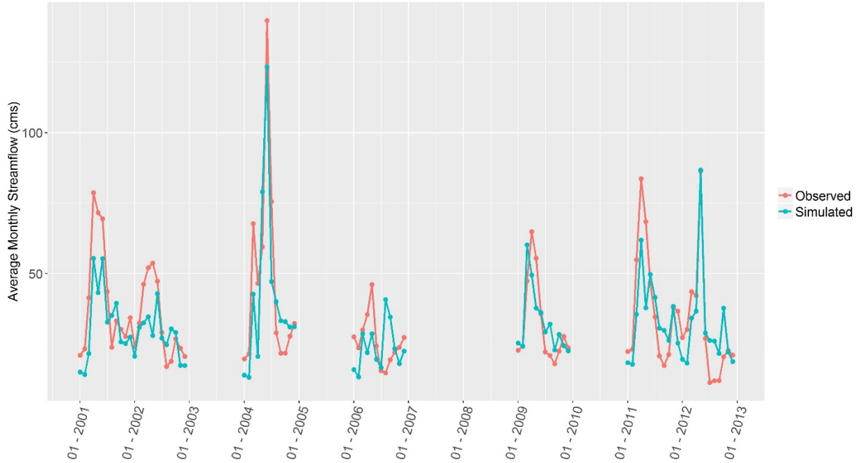
Figure D- 11. Monthly streamflow calibration hydrograph for USGS site 04073500 (Fox River at Berlin, WI).
