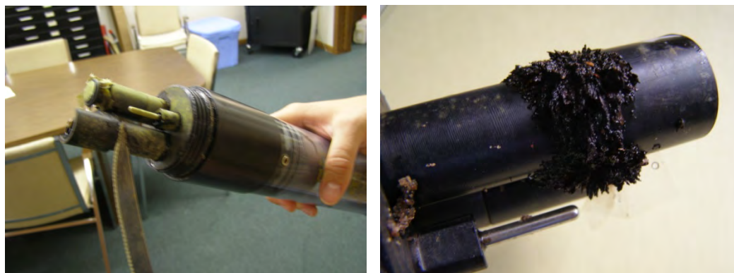
Pictured above: Typical two week accumulation of biofouling and iron filing accumulation of the Power Dam unit seen late-June and July.
