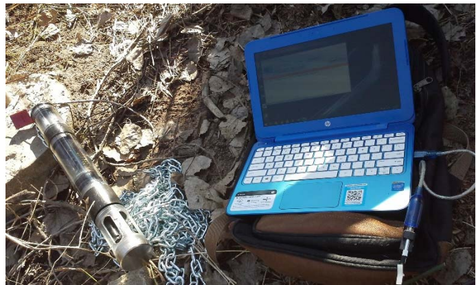
Data logger connected field computer during data download event.
