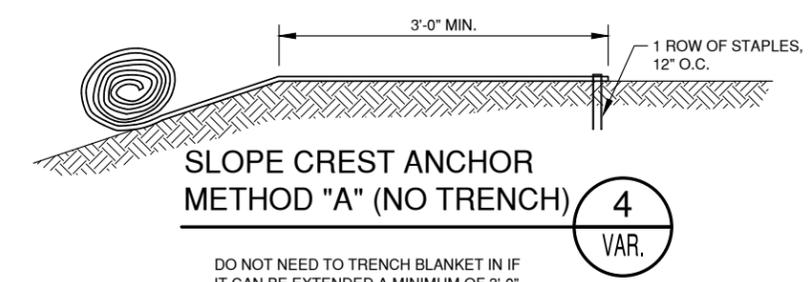
**SLOPE CREST ANCHOR METHOD "A" (NO TRENCH)** 4
