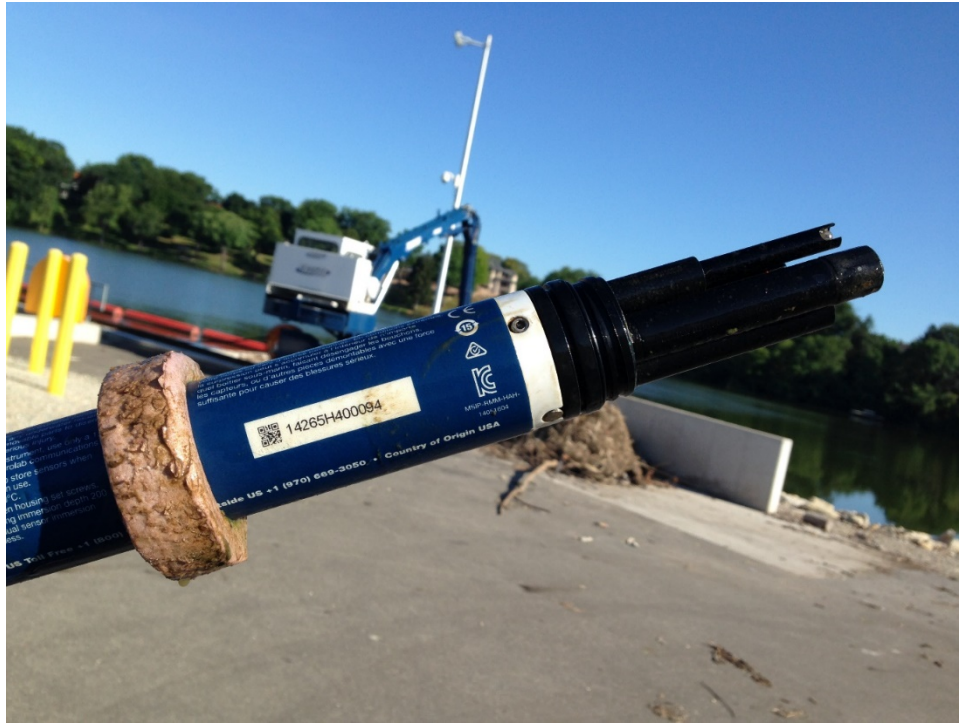
Photo No. 1 Example of moderate biofouling of sonde at Badger Upstream (8/8/16).
