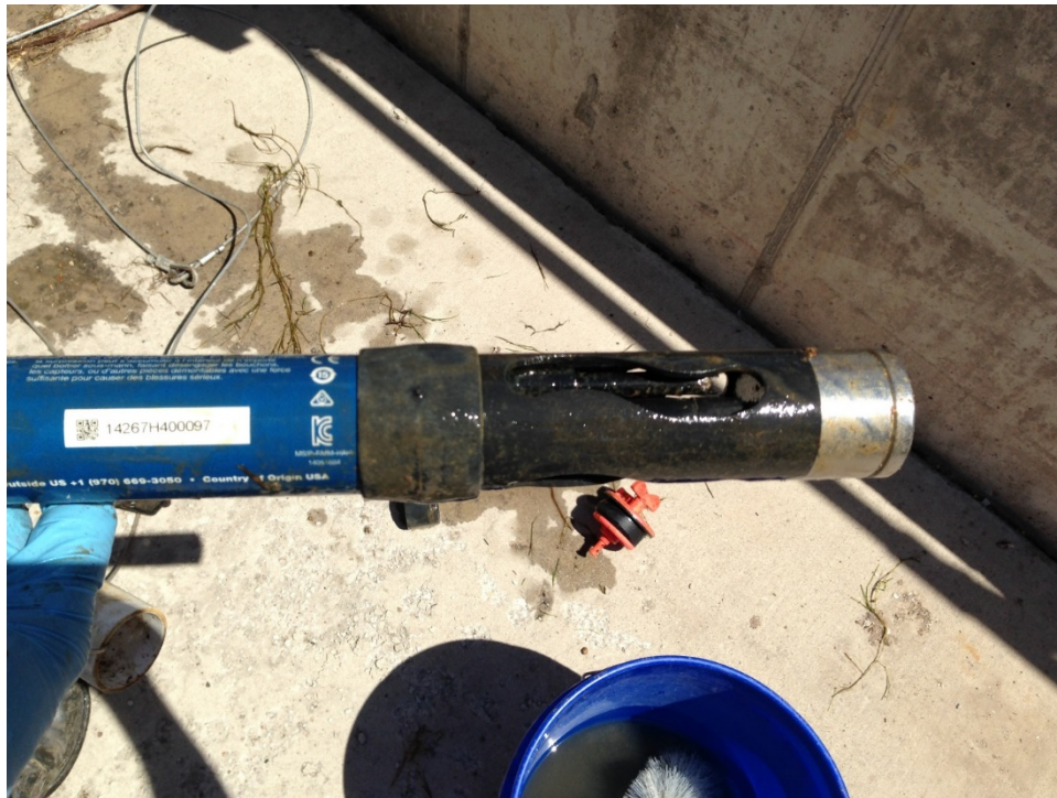
Photo No. 2 Example of sonde biofouling at Badger Downstream (8/8/16).
