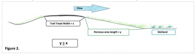
d. The pervious area must receive runoff in a sheet flow (as opposed to concentrated flow) manner across an impervious area with a pervious width at least as wide as the contributing source area (i.e., trail tread width). (Figure 3.)
