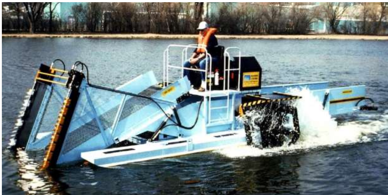
Figure 33 – Aquarius Systems EH-220 Aquatic Plant Harvester with a 5-ft cutting blade and 210 cu.ft cut material storage
