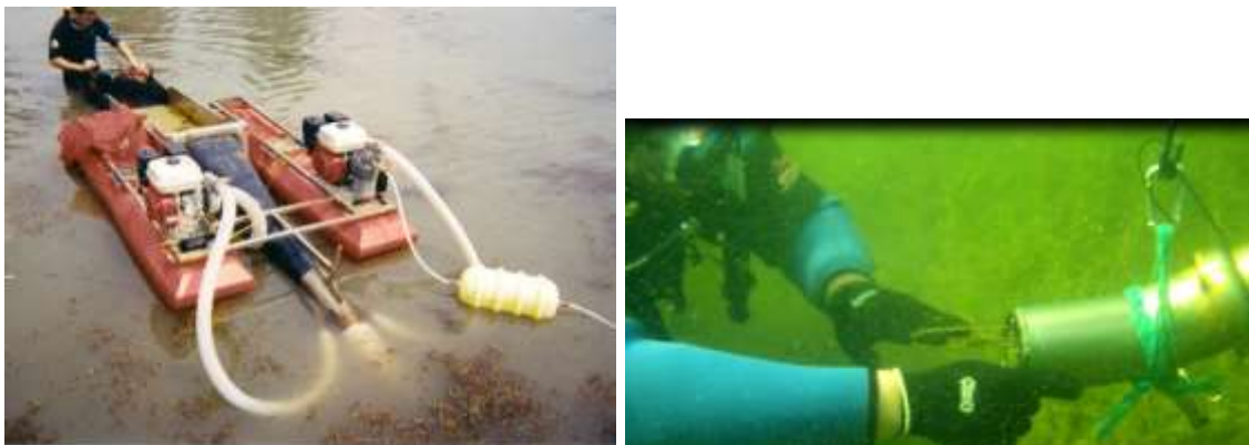
Figure 29: DASH - Diver Assisted Suction Harvest (Aquacleaner Environmental, http://www.aquacleaner.com/index.html ); Many Waters, LLC)
