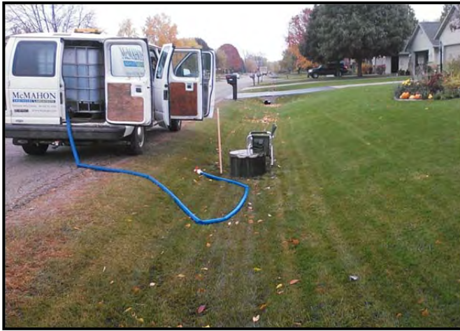
Double-Ring Infiltrometer Test
