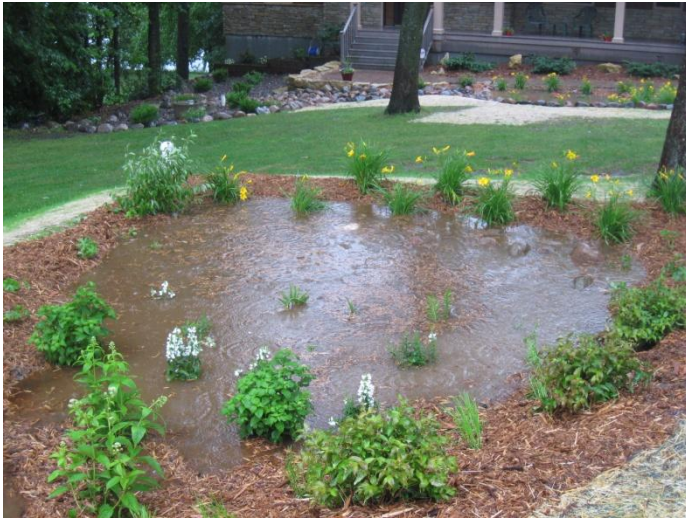
Figure 18. Rain Gardens Collect and Infiltrate Runoff Water (photo by Steve Palmer)
