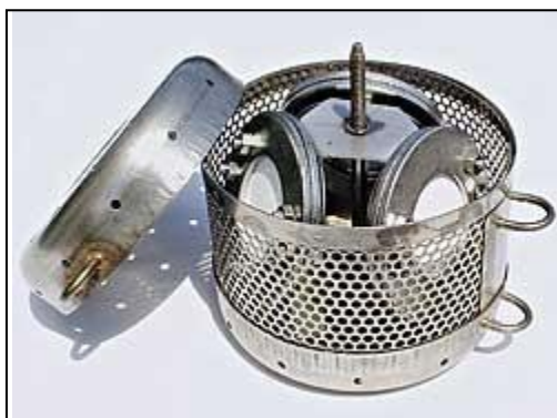
FIGURE 27. POCIS devices (discs with white centers) shown mounted in a deployment canister. Note: In the figure, three POCIS are mounted, whereas this study deployed one POCIS per canister. (Source: www.est-lab.com/pocis.php )
