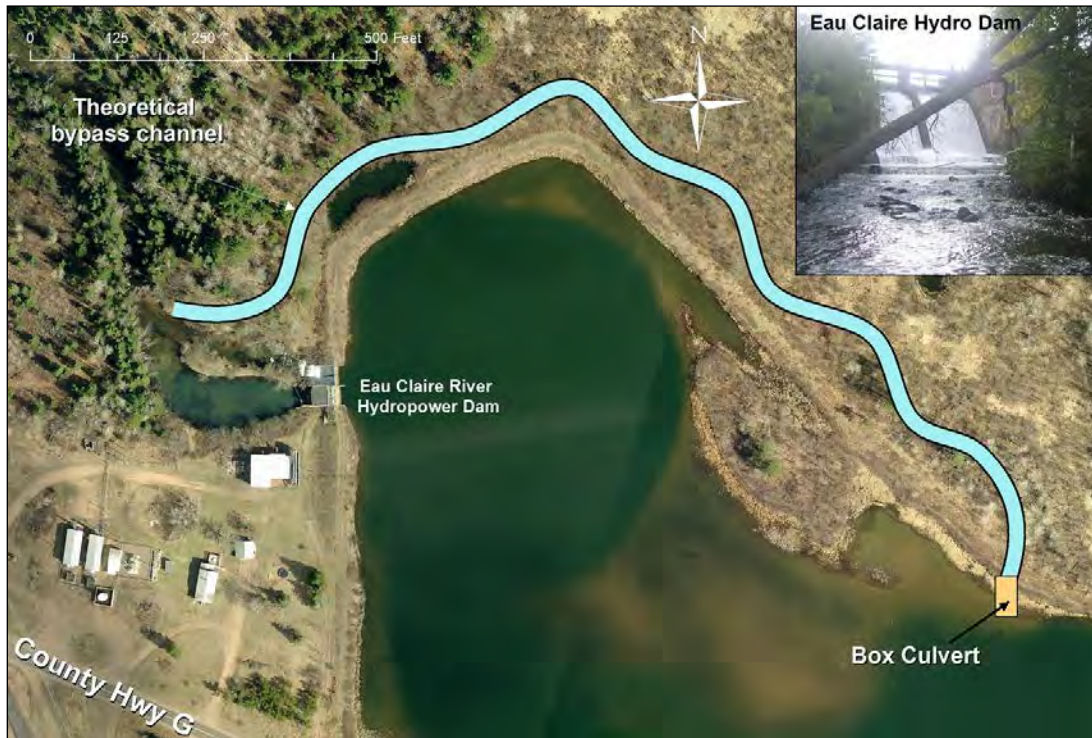
Figure 26 - Conceptual plan for fish passage at the Eau Claire Hydropower dam via a bypass channel.
