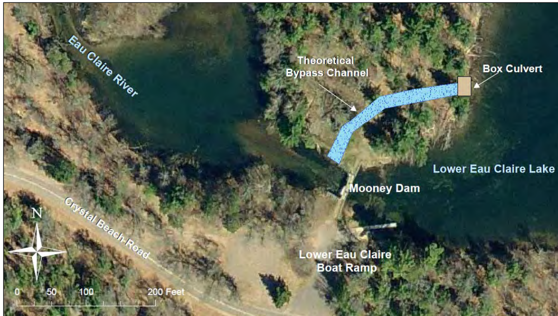
Figure 29 - Conceptual plan for fish passage at Mooney Dam via a bypass channel.
