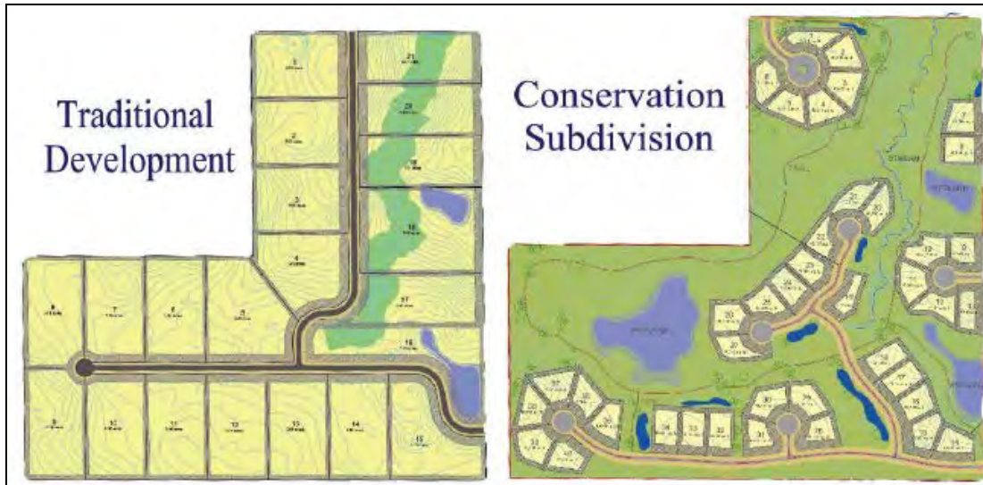
Figure 43 - An example of a conservation subdivision design from Walworth County, WI. Minimum lot sizes were reduced, but design allowed for 70 acres of common open space, the protection of a stream corridor, and natural stormwater management.
