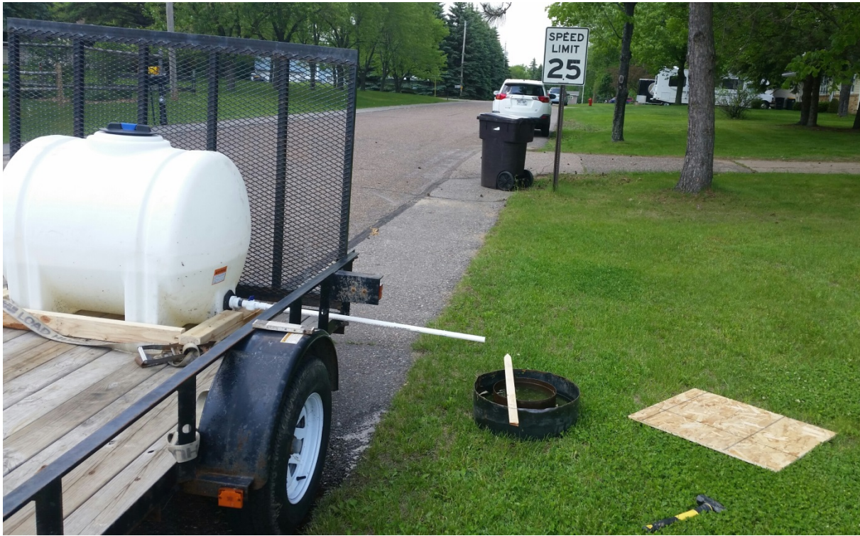
Double-ring infiltrometer test apparatus with water tank.
