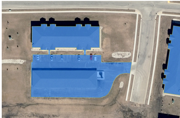
An aerial photograph outlining impervious surfaces on a commercial property.
