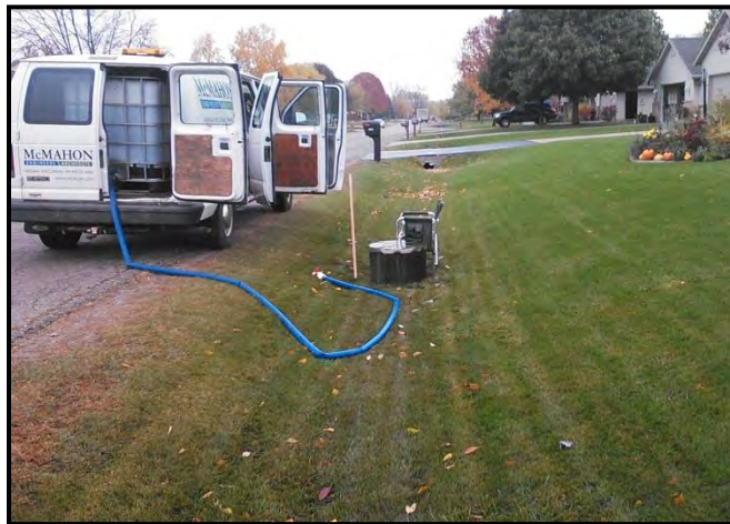
Double-Ring Infiltrometer Test
