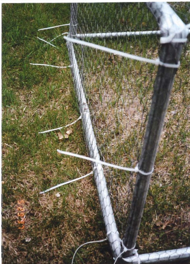
Figure 2. A total of eighteen enclosures were placed in Cedar Lake. An example of an enclosure is shown above. Chicken wire was attached to the 1-inch diameter conduit with cable ties (bottom photo).
