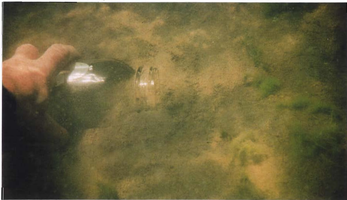
Figure 5. (Top) Recording sonar tracings show the areas where the exclosures were placed in deeper water. The seven foot depth on Jerry's transect (top, left) was not as steep as the seven foot depth at Jack's transect (top, right). (Bottom) Invertebrate samples were collected using a glass jar and collecting sediments to a depth of 8 cm (3 inches).
