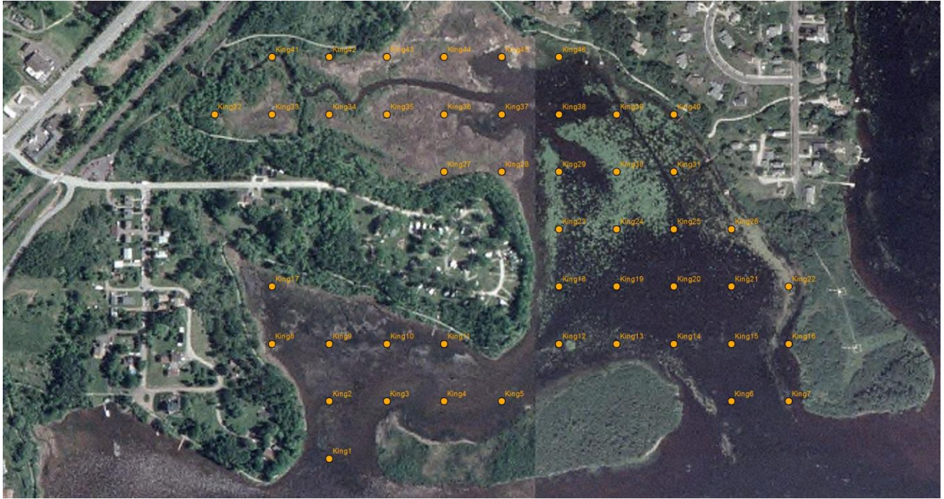
Figure A-13: Monitoring Points in Kingsbury Bay (46 points, 80 m grid) (several points in north part of bay inaccessible in 2017 due to bog/cattail, potential open water in future after planned restoration work)
