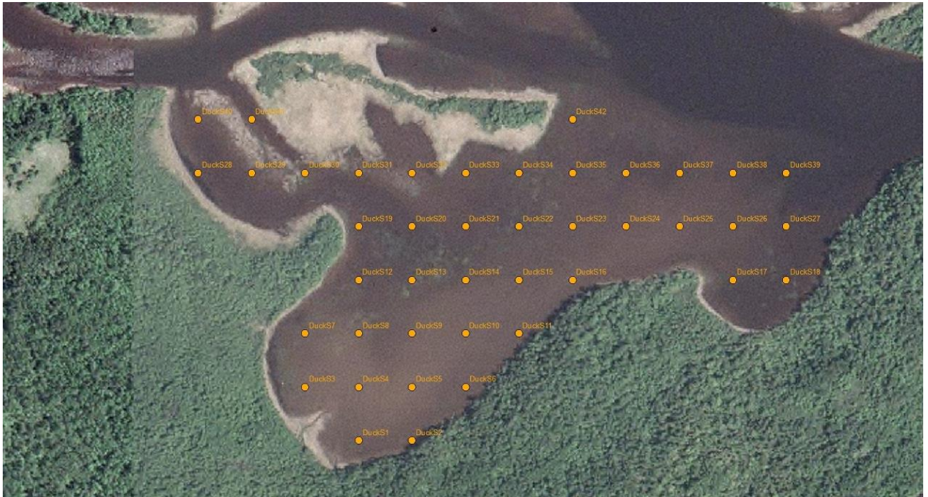
Figure A-3: Monitoring Points in Duck Hunter Bay south (42 points, 75 m grid)
