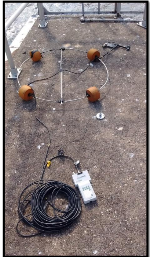
LI-COR sampling equipment used to measure underwater light.
