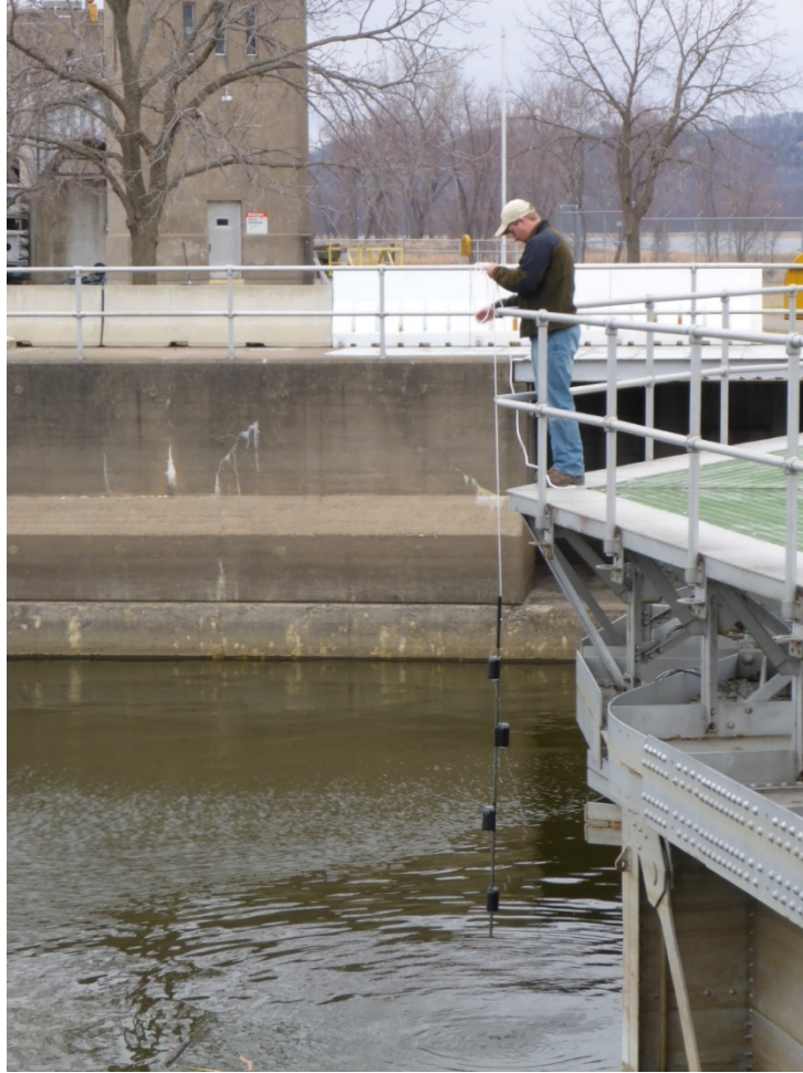
Figure 2. Example of sediment trap deployment at Lock and Dam 3. The traps are lowered below the water surface for roughly 60 days of passive sampling.
