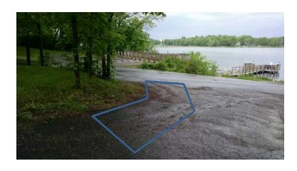
Here is another area where underpavement infiltration could be installed. A diversion (trench or asphalt bump) would be needed to get water to this spot.
