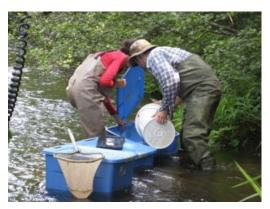
stream's physical characteristics were determined by examining a cross-section every five meters. Water flow was measured, the stream width was measured, and the composition of the stream bottom was analyzed. In addition, the tree canopy was measured, the water temperature was recorded at multiple locations, photographs were taken, the amount of wood in and along the stream was determined, and the elevational change of the 100 meter section was measured.
