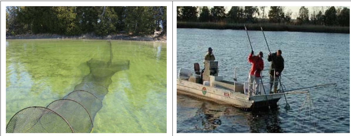
Photo 8.4.6-1. Fyke net positioned in the littoral zone of a Wisconsin lake (right) and an electroshocking boat (left).
