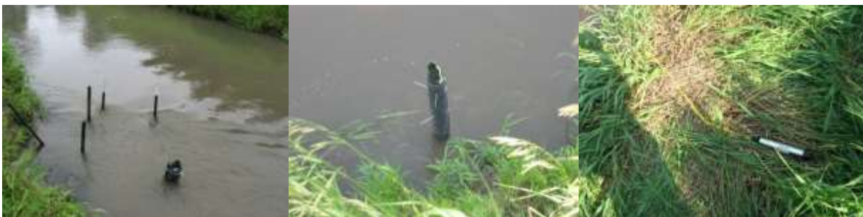
Figure 11 – Installation of pressure transducers (data logger) to measure depth of water (Papanicolaou, 2017)
