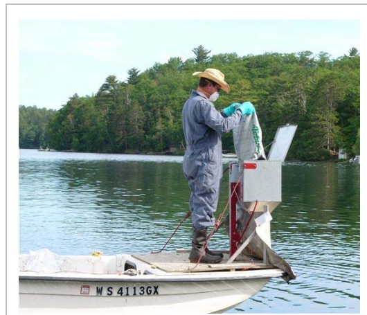
Photograph 3.4-4. Herbicide applicator. Applying granular herbicides with a gravity-fed dispersion method.
