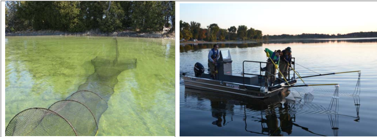
Photo 3.5-1. Fyke net positioned in the littoral zone of a Wisconsin Lake (left) and an electroshocking boat (right).
