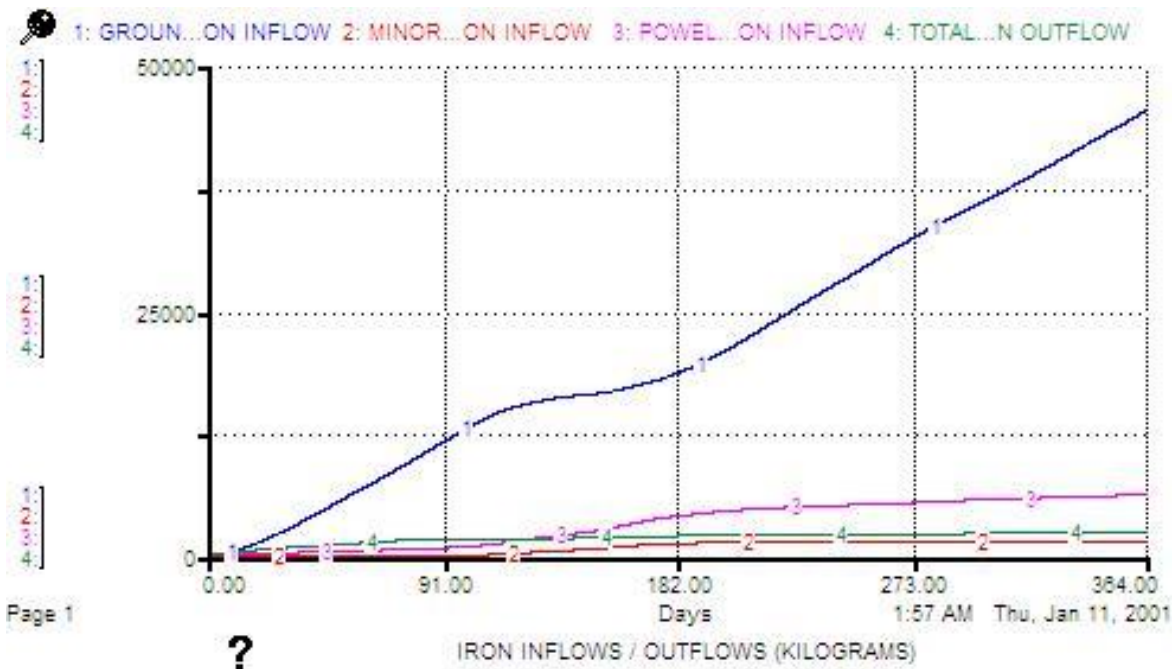
STELLA GRAPH 3. The total accumulated iron load to Dead Pike Lake starting in April 2017. The Blue line (#1) represents the iron groundwater load. The Red line (#2) represents the iron load from Pete's and Deerfoot Marsh creeks. The Purple line (#3) represents the iron load from Powell Marsh. The Green Line (#4) represents the iron load leaving Dead Pike Lake.
