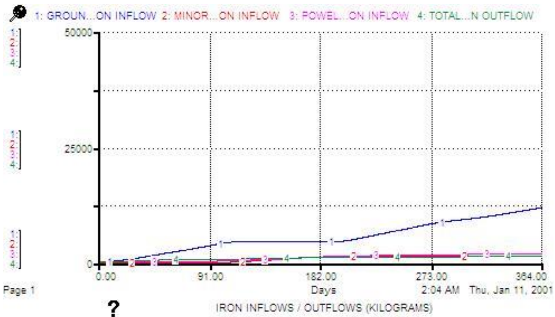
STELLA GRAPH 4. This graph models the difference from GRAPH 3 with a 1 foot increase in the elevation of the Dead Pike Lake outlet stream and a wetland biofilter system in Powell Marsh. The Blue line (#1) represents the iron groundwater load. The Red line (#2) represents the iron load from Pete's and Deerfoot Marsh creeks. The Purple line (#3) represents the iron load from Powell Marsh. The Green Line (#4) represents the iron load leaving Dead Pike Lake.
