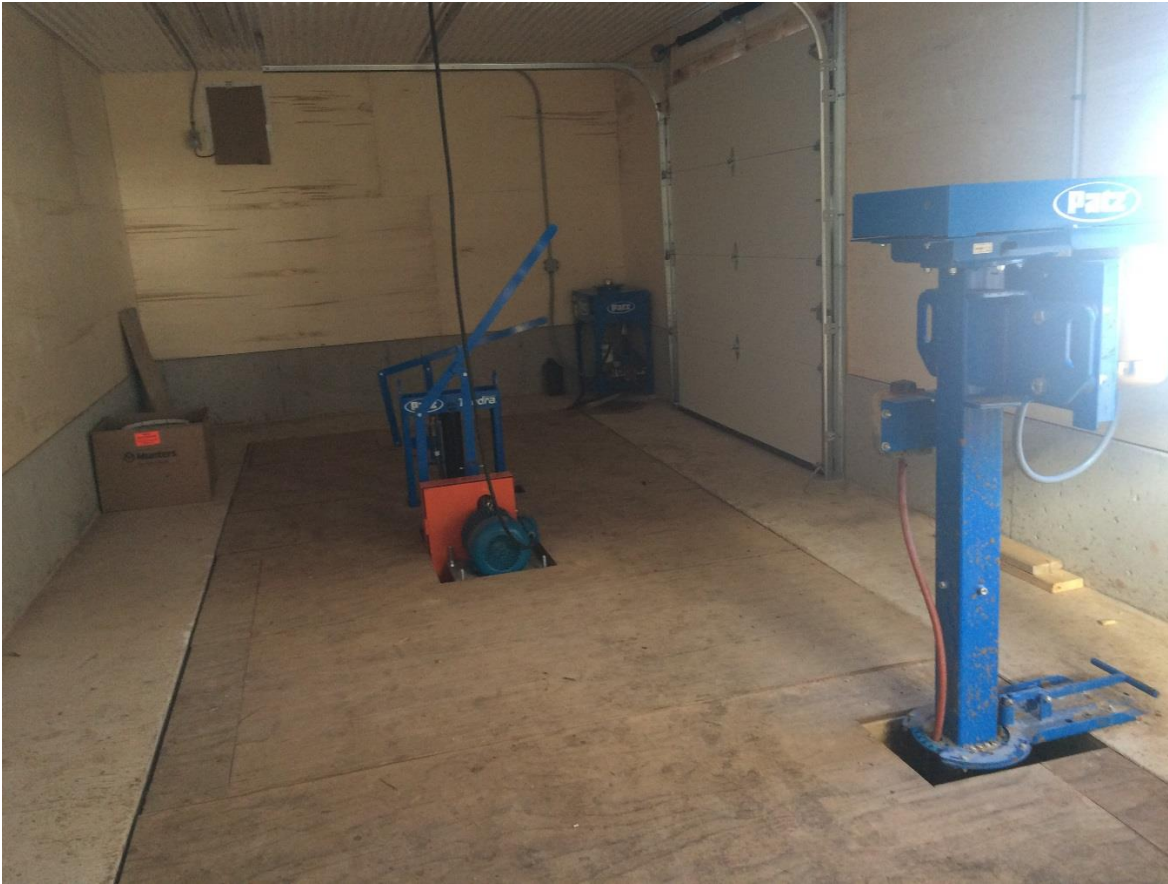
Waste Transfer – 18" Auger Channel with sand auger & slatted grating
