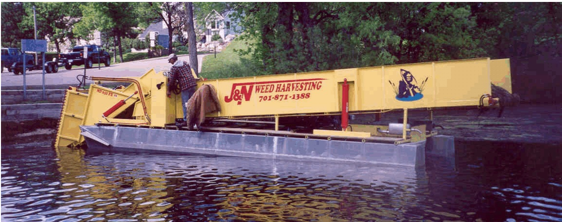
Figure 27. A mechanical harvester is recommended for controlling nuisance milfoil growth in open water.
