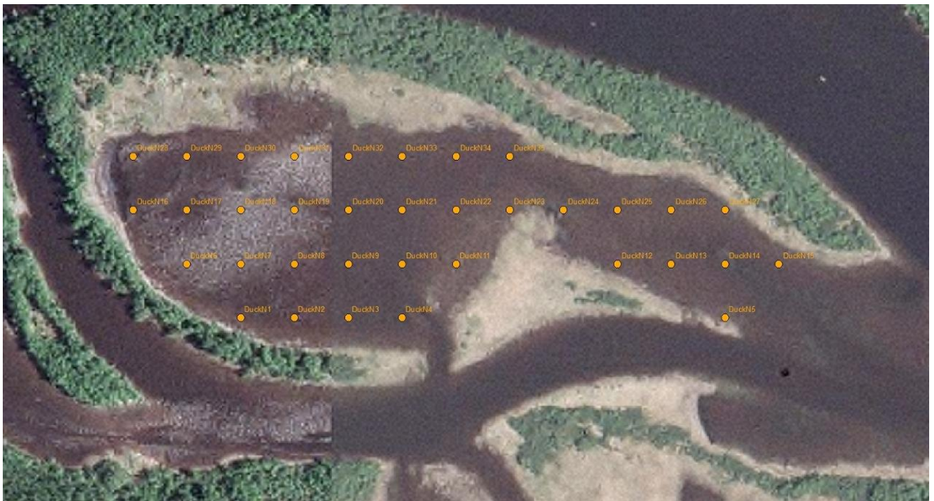
Figure A-2: Monitoring Points in Duck Hunter Bay north (35 points, 50 m grid)
