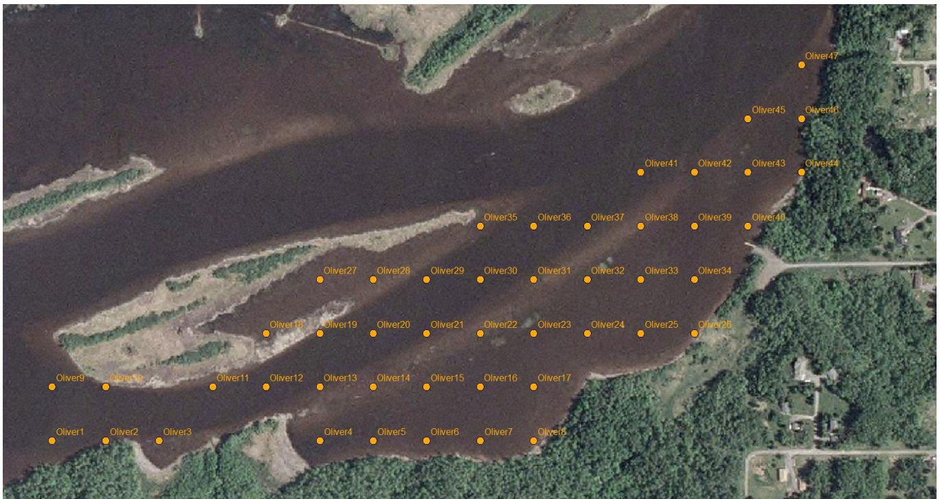
Figure A-8: Monitoring Points in Oliver-Bear Island (47 points, 75 m grid)
