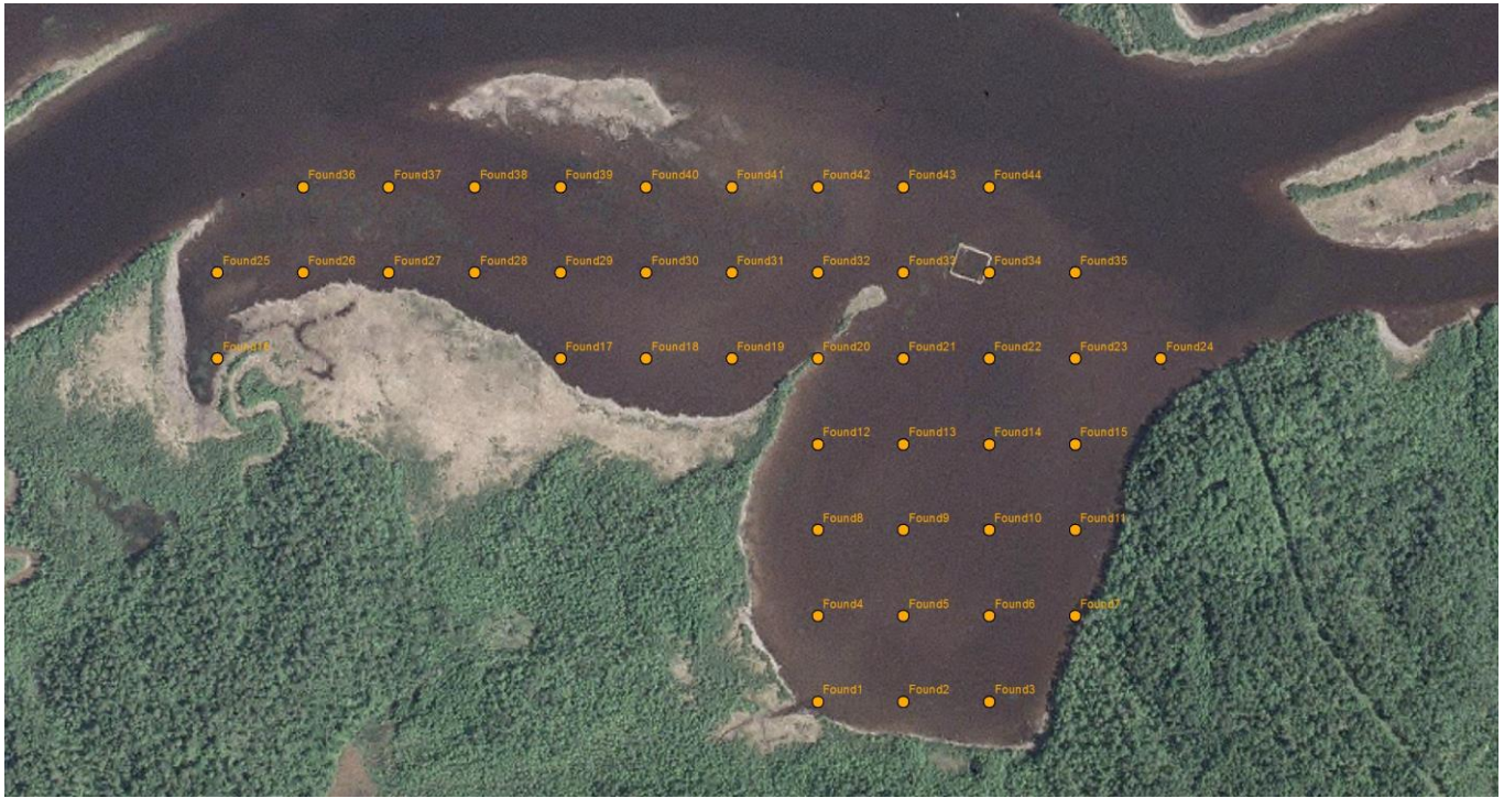
Figure A-11: Monitoring Points in Foundation Bay (44 points, 100 m grid)
