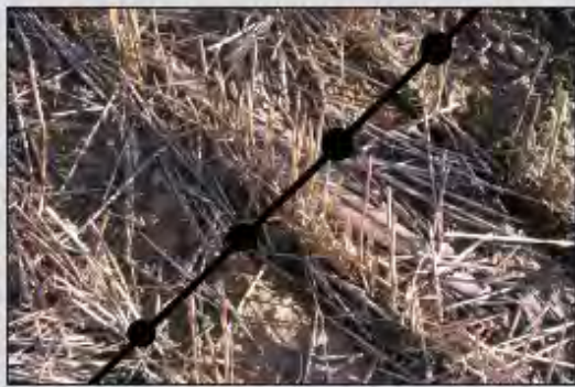
Illustration of line-transect method for residue.
