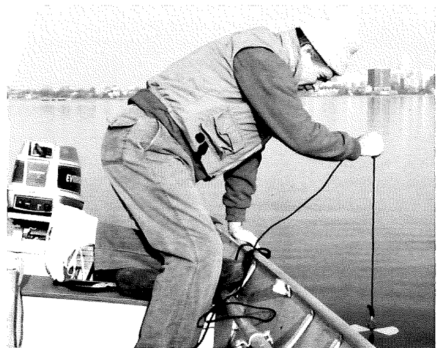
DNR's Dick Lathrop measuring water clarity in Lake Monona with secci disk.
