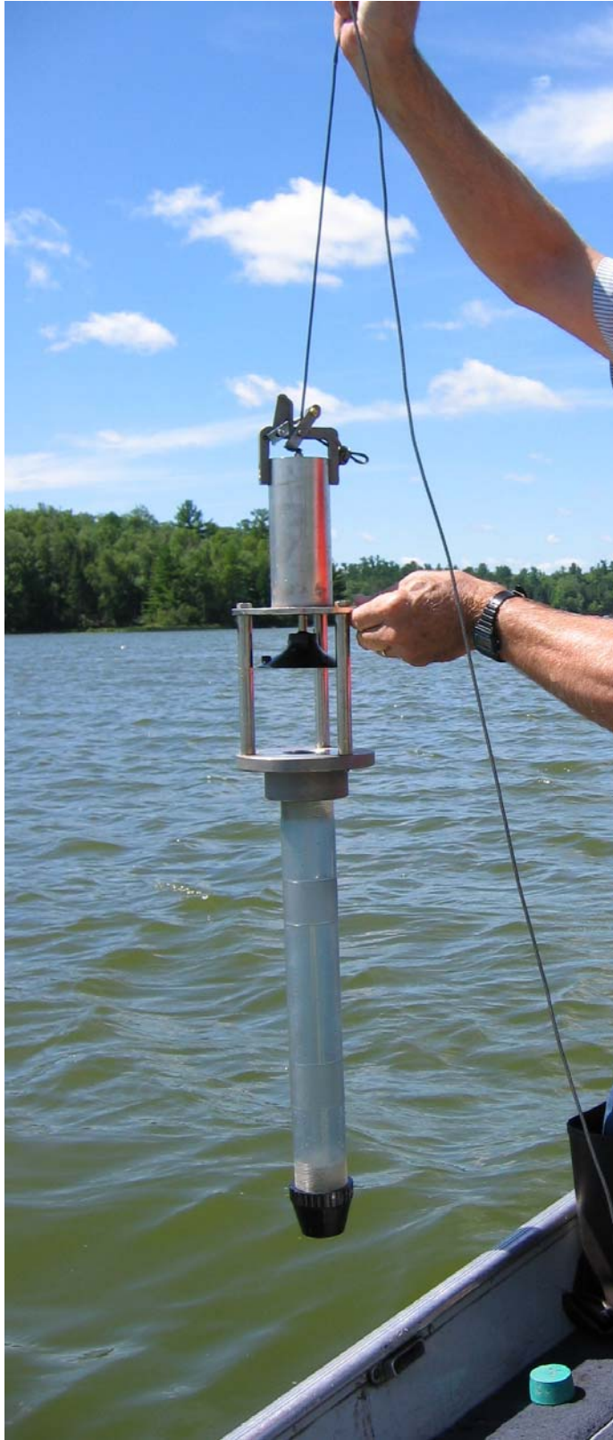
Figure 2. Core sampler readied for lowering into lakebed of Butternut Lake.
