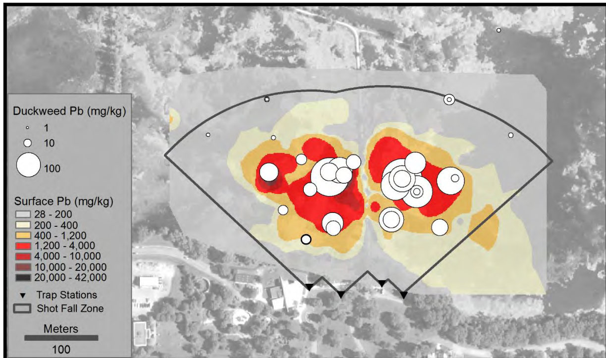
Figure 15. Location of UWL duckweed sampling sites. Sites are identified on top of spatially interpolated surface (0-5 cm) Pb concentrations in LRM sediments. Circle size is proportional to concentration of Pb in duckweed tissue (mg/kg dry mass).
