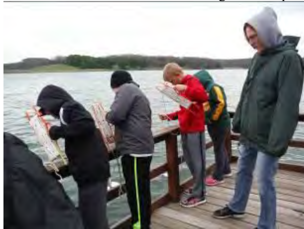
Using Secchi disk to measure water clarity
