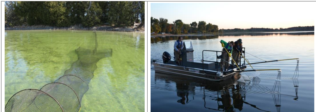
Photograph 3.6-1. Fyke net positioned in the littoral zone of a Wisconsin Lake (left) and an electroshocking boat (right).
