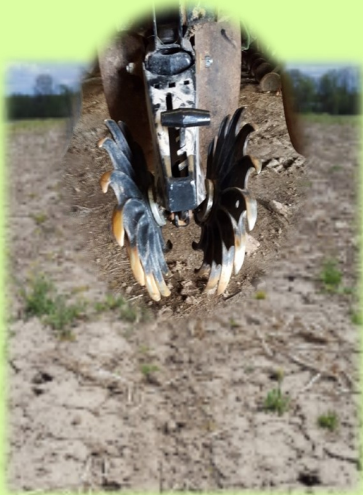
Figure 1: Field was planted with Dawn Curvtine closing wheels. Note the loose soil covering the seed furrow (Dawn Curvtine results: 34,000 pp).
