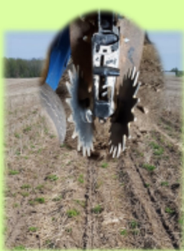
Figure 2: Field was planted using Extapa closing wheels. Note the defined seed furrow (Extapa results: 32,571 pp).
