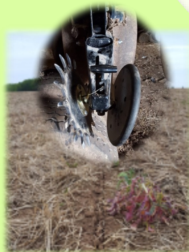
Figure 3: Field was planted using a Martin + Smooth seed closing combination. Note the defined seed furrow (Martin + Smooth results: 33,857 pp).
