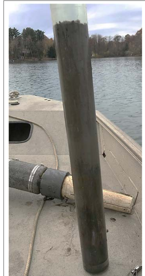
Photograph 3.2-2. Photo of sediment core collected from Stratton Lake. There were several color changes below 42 cm.
