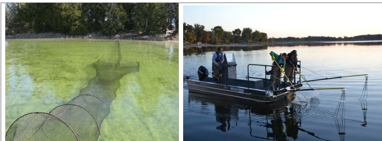
Photograph 3.7-1. Fyke net positioned in the littoral zone of a Wisconsin Lake (left) and an electroshocking boat (right).
