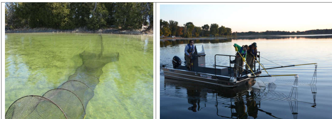
Photograph 3.7-1. Fyke net positioned in the littoral zone of a Wisconsin Lake (left) and an electroshocking boat (right).
