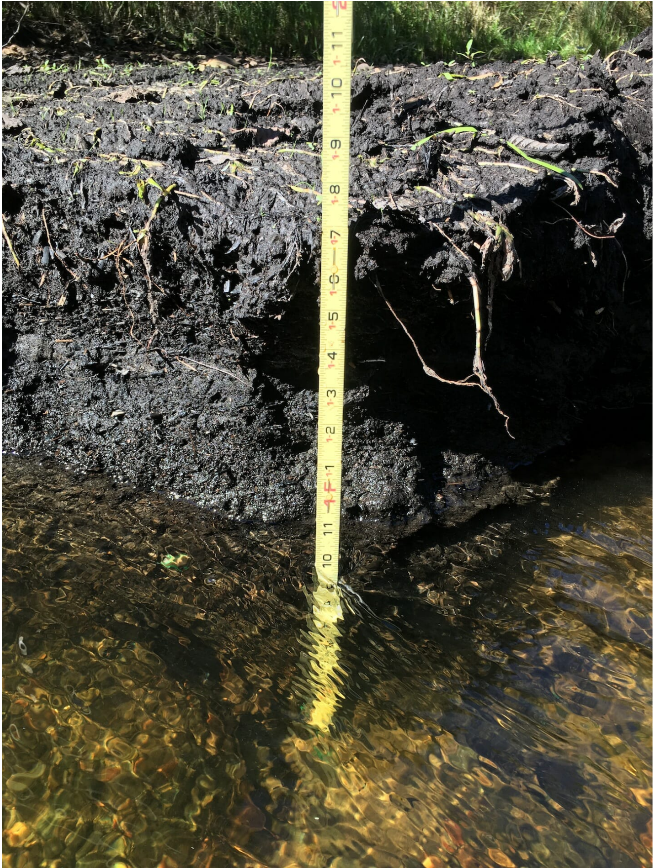
The average width and depth of the channel were both reduced to natural conditions mimicking the upstream and downstream reference reaches.
