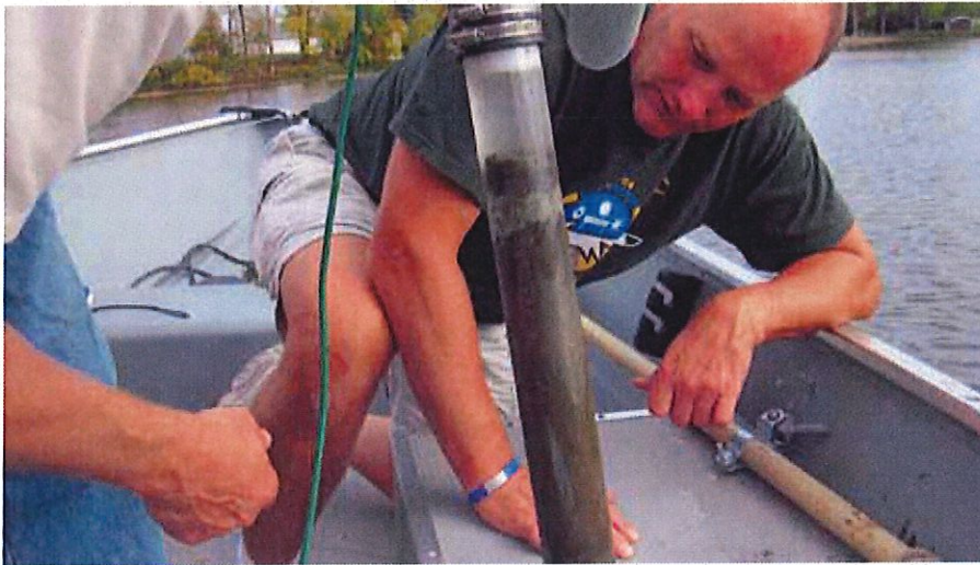
Figure 7. Bottom core extracted from the deepest location in East Alaska Lake approximately one year after the alum treatment. The white section is the alum layer that has settled approximately two inches into the soft bottom sediments.
