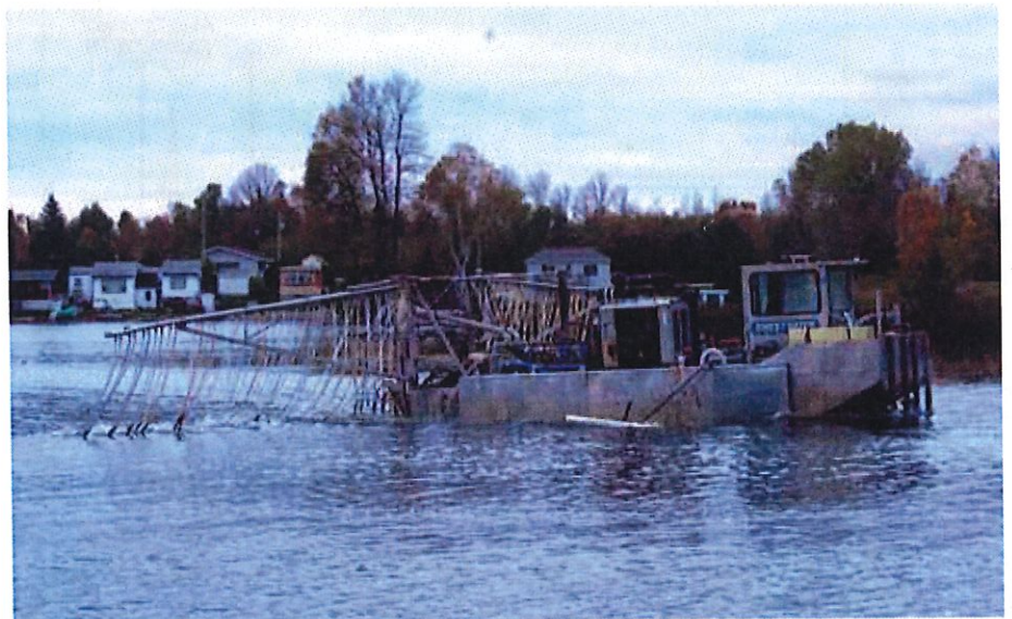
Figure 3. Barge applying alum to East Alaska Lake during October 2011.
