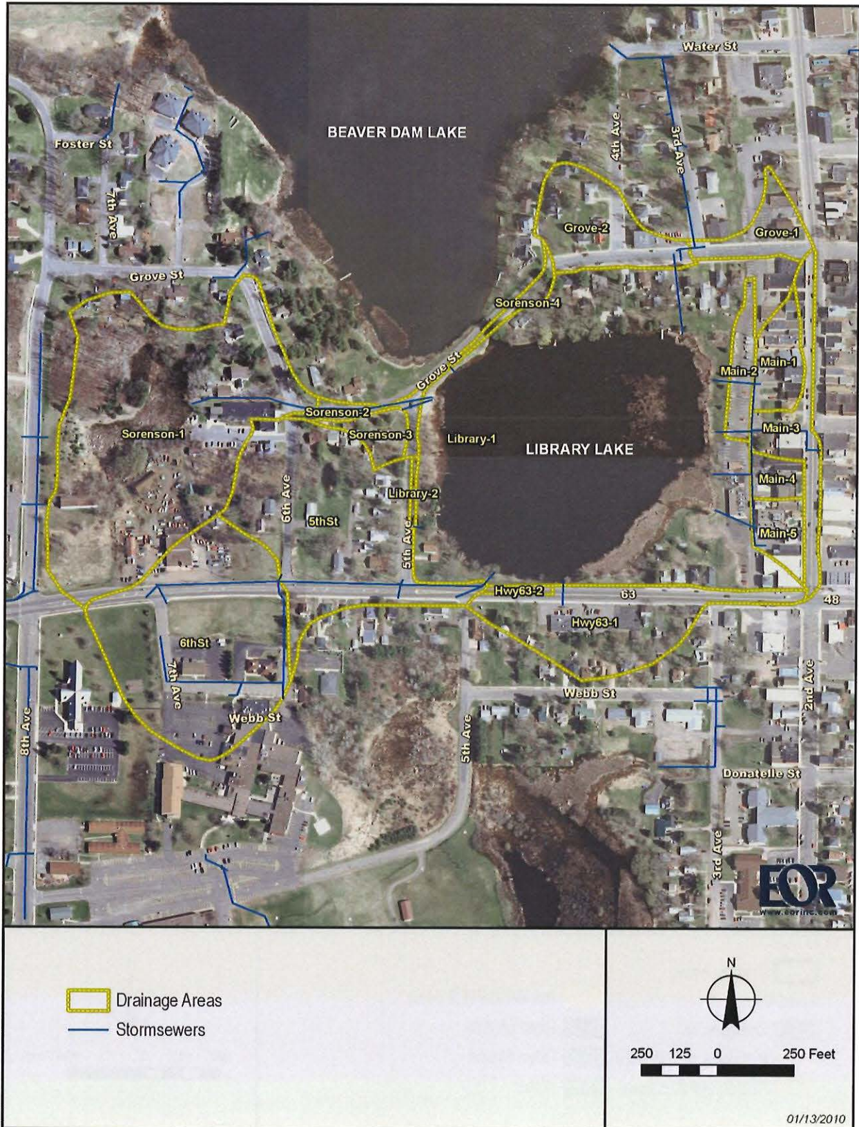
Figure 4. Drainage Areas with Stormsewers Indicated
