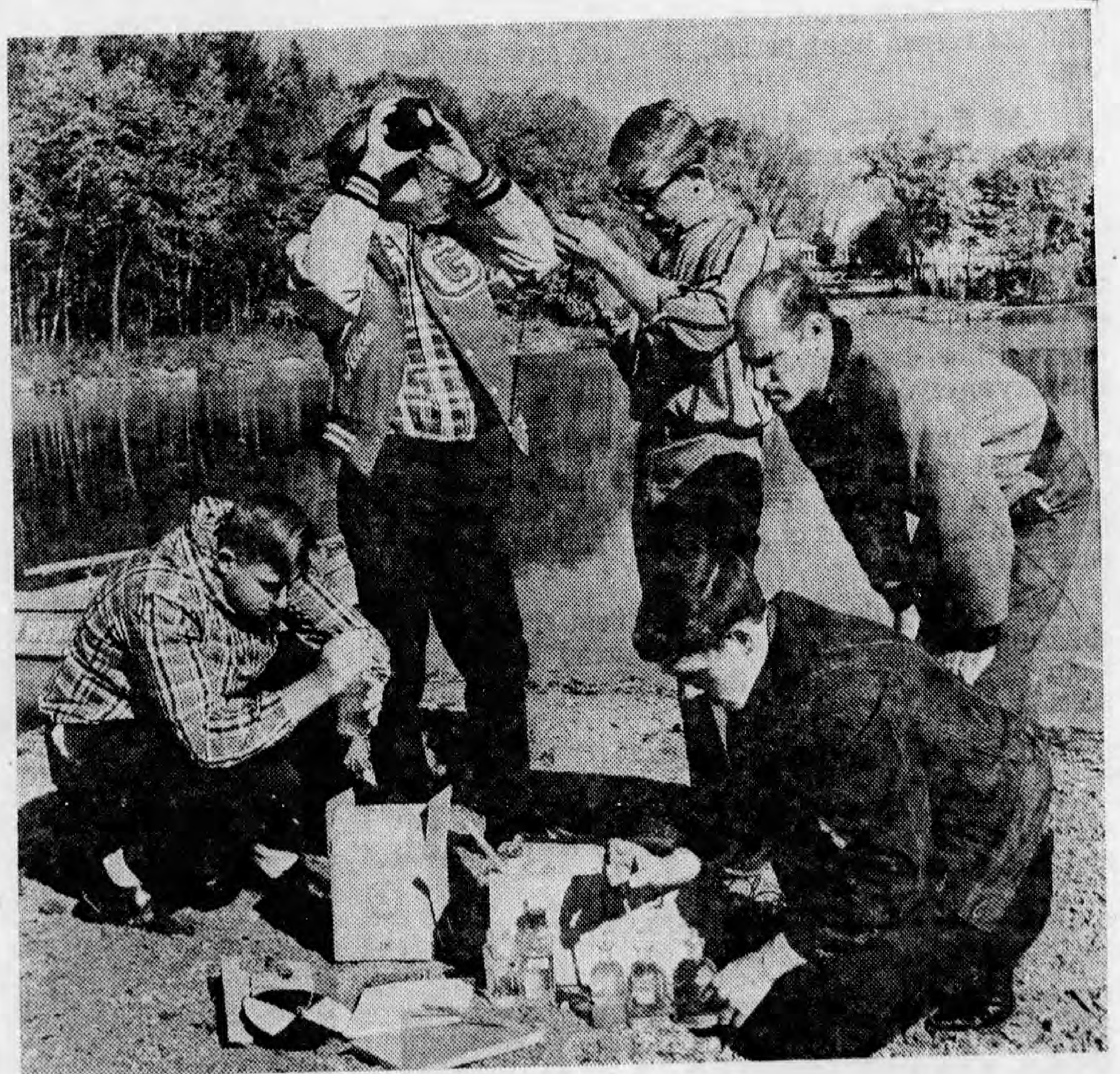
SAMPLES SUBJECTED TO TESTS Students prepare samples for oxygen tests, take alkalinity readings and temperatures
