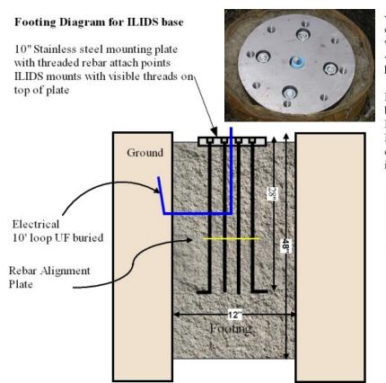
4- 5/8" threaded rods come thru footing plate which is fastened with 4 nuts in countersunk holes so face is flush.
