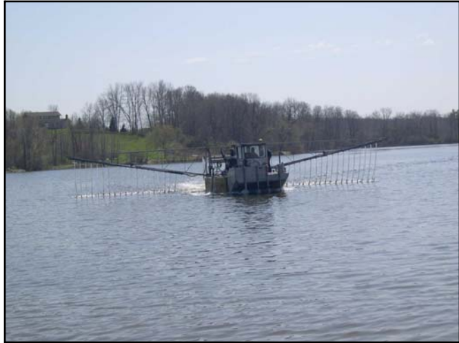
Figure 11. Picture of the barge applying alum to reduce phosphorus release from the deep water sediments.
