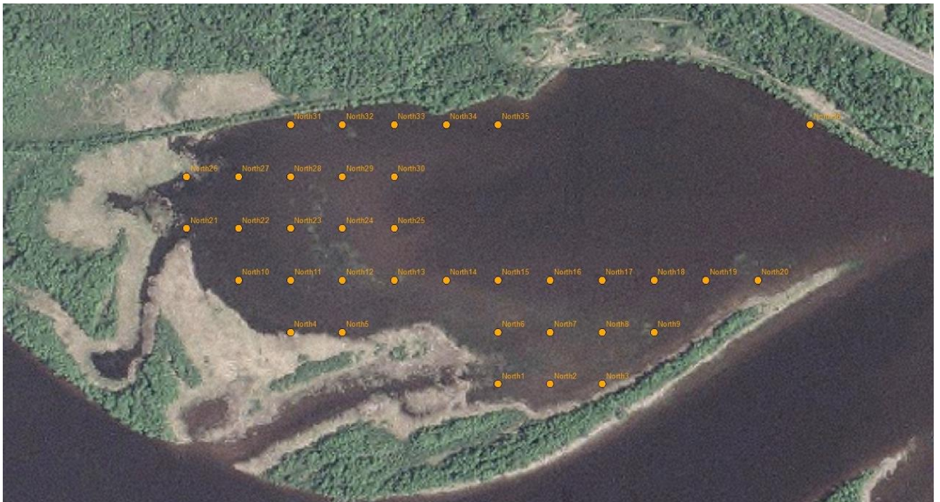
Figure A-4: Monitoring Points in North Bay (36 points, 60 m grid)
