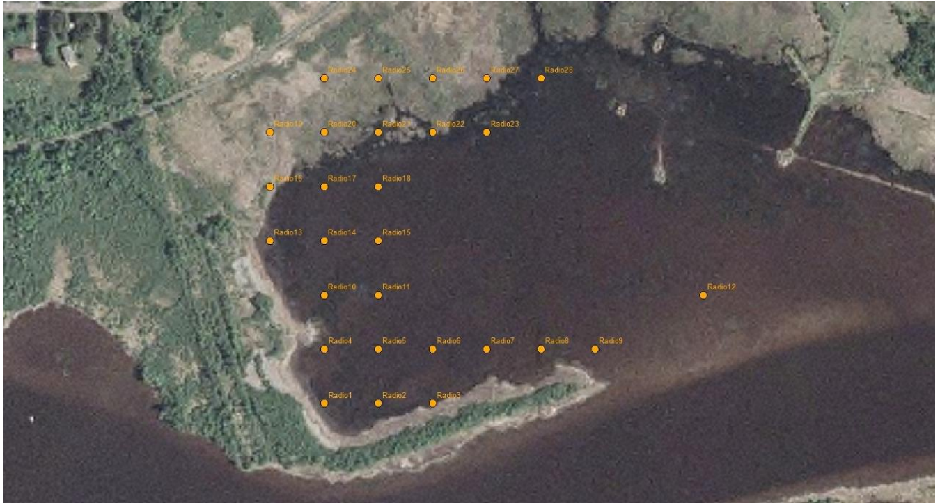
Figure A-5: Monitoring Points in Radio Tower Bay (28 points, 50 m grid) (aerial photograph taken before open water habitat created in north portion of bay)
