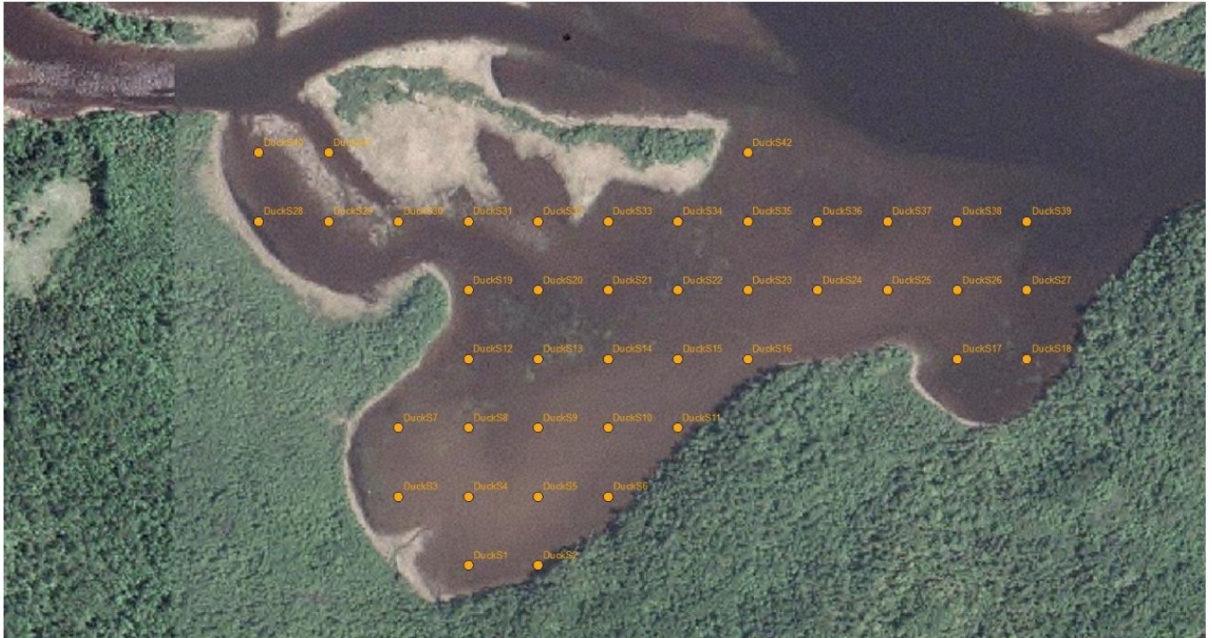
Figure A-3: Monitoring Points in Duck Hunter Bay south (42 points, 75 m grid)
