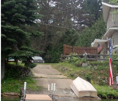
Figure 15. Impervious surfaces and straight trail/road access allow runoff to speed up and brings phosphorus laden sediments to the lake. This site (not on Pioneer Lake) was augmented with a water infiltration pit to minimize runoff going into the lake.
