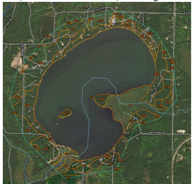
Figure 3. Soils of Pioneer Lake. Seelyeville and Markey mucks (Se), Sayner-Rubicon complex (SaC & SaD), Rubicon sand (RoB), Croswell sand (CrA), and predominate the riparian area. Courtesy Soil Web Survey, NRCS.
