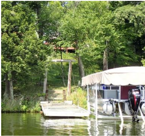
Figure 8. Minimizing impervious surfaces in and around lake access paths, maintaining vegetation, and curving the trail across the slope keeps shoreland erosion in check.
