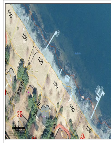
Arial view showing planting area in red. Yellow Line is 1222'. OHWM is 1221.8'
