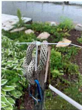
6/21/19. Caribener with eyelet from curtain and plastic zip ties that were used to secure curtain, ripped out of curtains.
