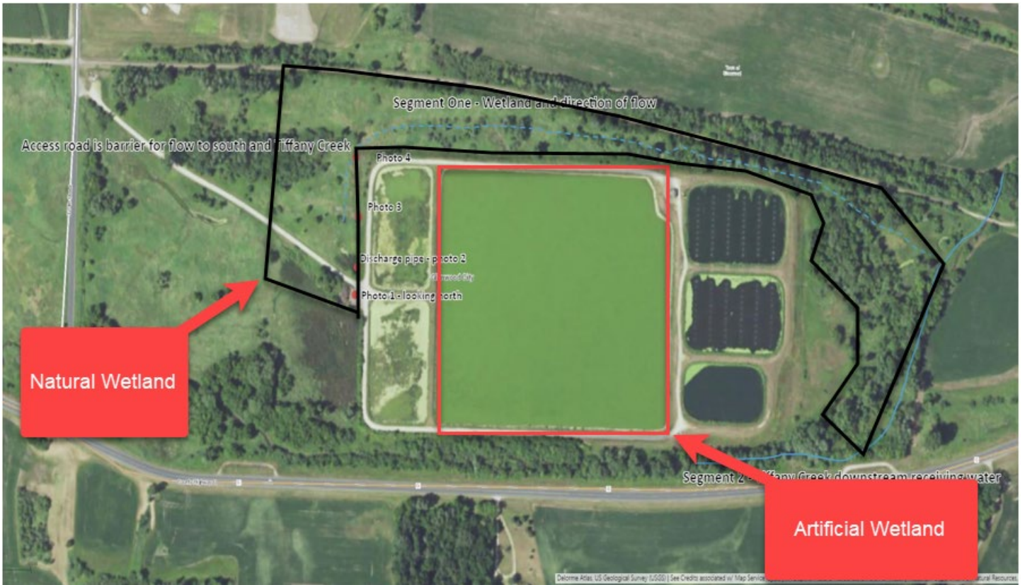
Figure 2 – Map showing the extent of the artificial wetland (red line) that is part of the treatment system, and the surrounding natural wetland that is the direct receiving water (black line).
