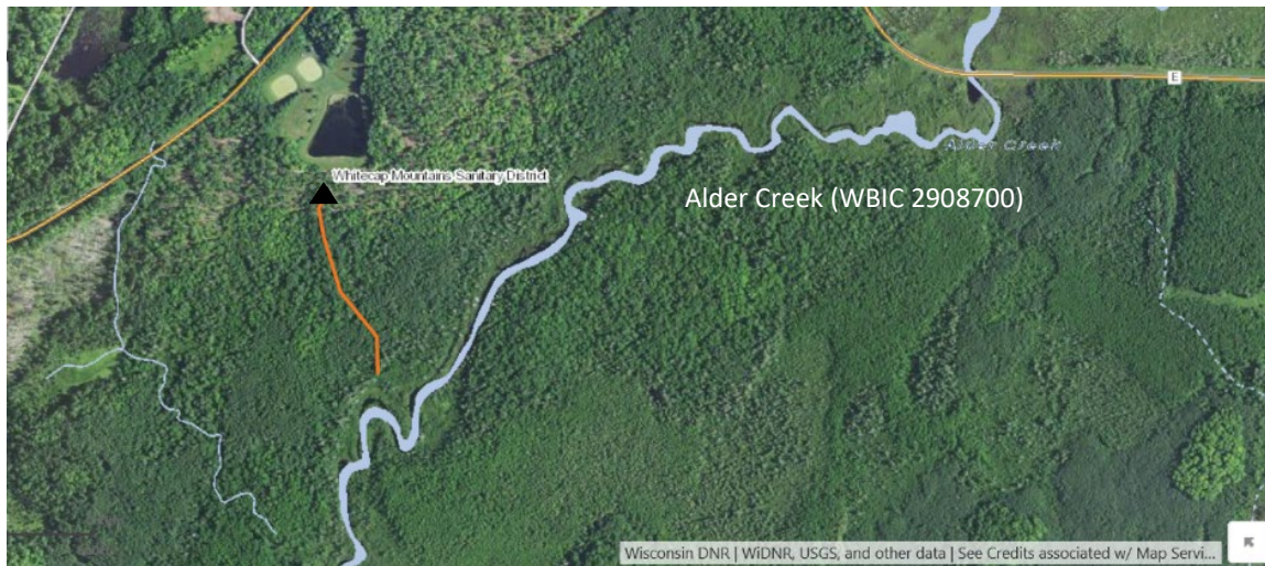
Figure 1. Aerial Photo Map: Orange line indicates flow path from facility outfall (black triangle) to Alder Creek.
