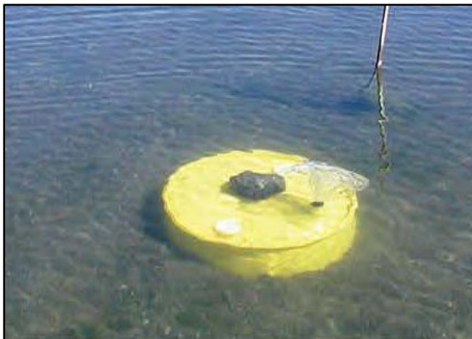
Figure 8. Seepage meters were constructed from 50-gallon plastic barrels.
